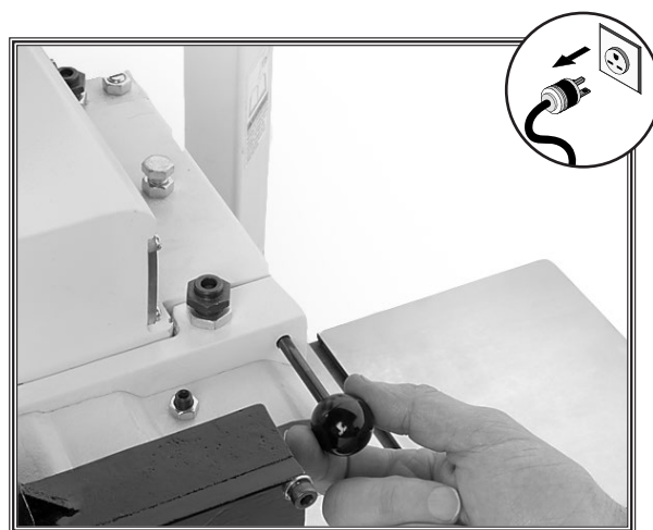
Figure 18. Removing chip deflector retaining pin.
