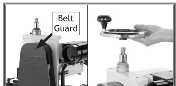
Figure 13. Belt guard and handwheel installation.
