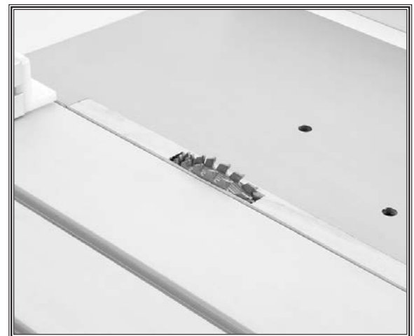
Figure 112. Dado blade raised into zero-clearance table insert.
