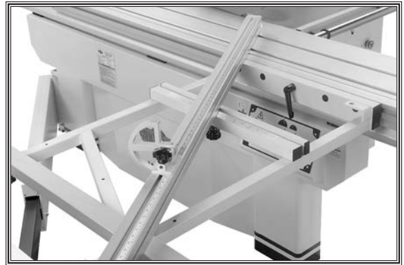
Figure 77. Fence set up for 90° to 135° cuts.
