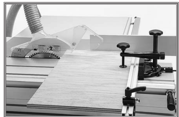
Figure 74. Crosscutting workpieces using the rip fence as a cut-off gauge.
