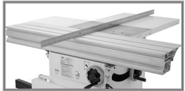
Figure 16. Extension wings mounted and even with cast-iron table.
