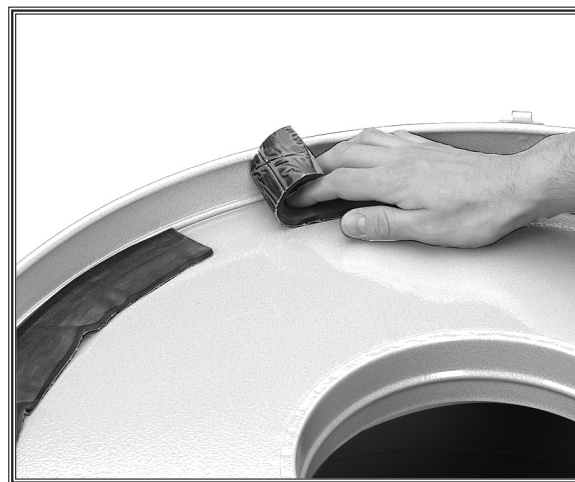
Figure 29. Attaching foam tape to collector drum lid.
