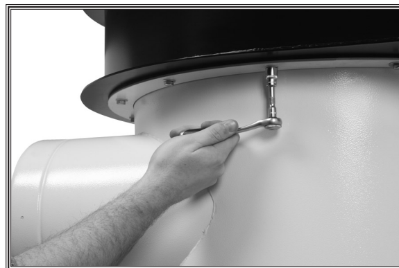
Figure 21. Securing intake barrel to blower.
