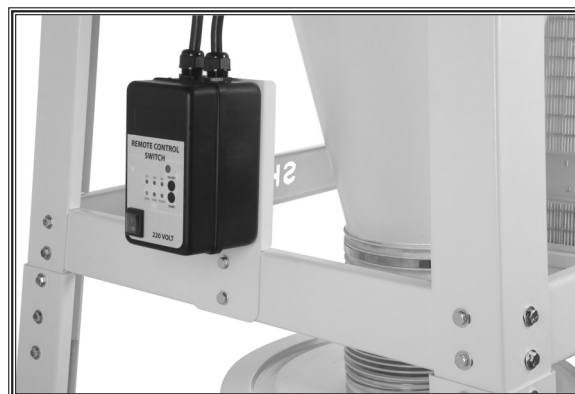
Figure 38. Switch mounted to stand.
