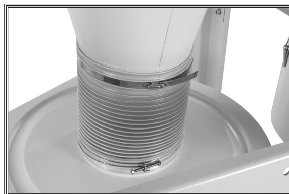
Figure 36. Drum attached to cyclone funnel with 9" hose clamps.
