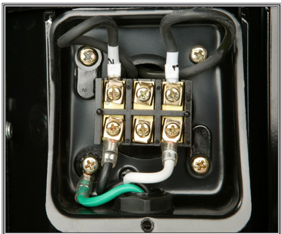
Figure 61. W1809 motor wiring.
