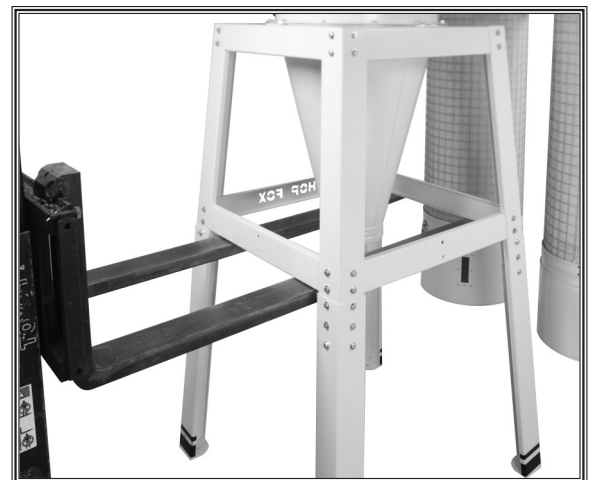
Figure 28. Lower stand legs attached (Model W1810).
