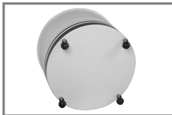
Figure 30. Casters attached to the lower collection drum.
