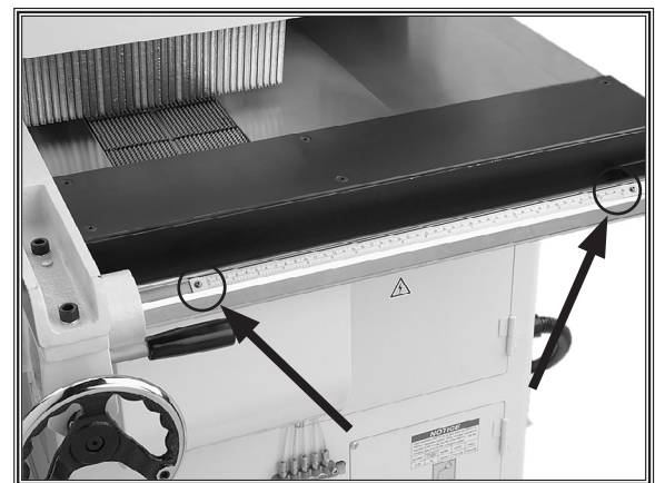
Figure 35. Location of screws securing the rip fence scale.
