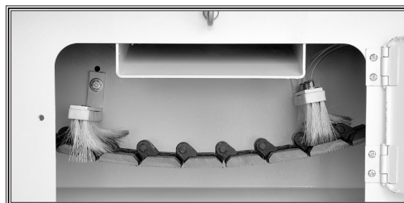
Figure 29. Conveyor track lubrication brushes.
