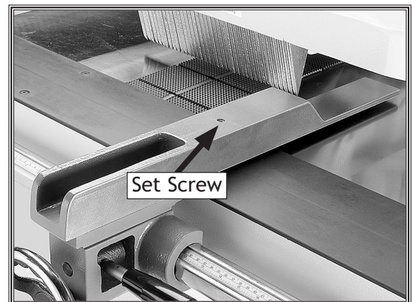
Figure 34. Fence ride height adjusting set screw.
