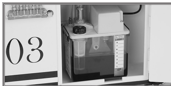
Figure 30. Lubricant system reservoir.
