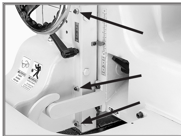
Figure 36. Location of headstock gib adjusting jam nuts and set screws.
