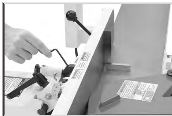
Figure 62. Adjusting fence to 90°.
