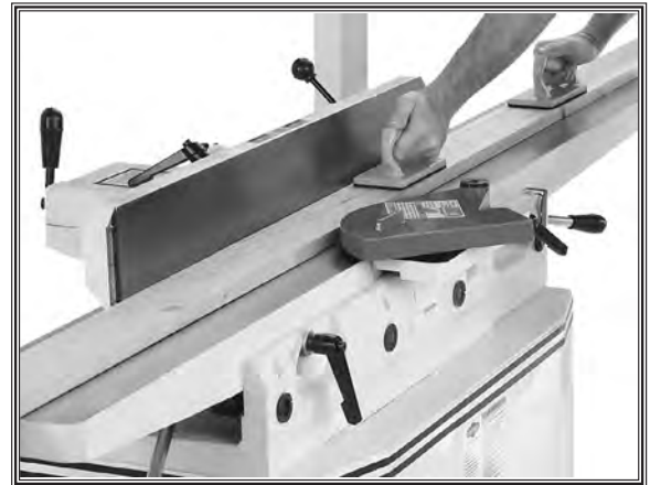
Figure 36. Typical surface planing operation.
