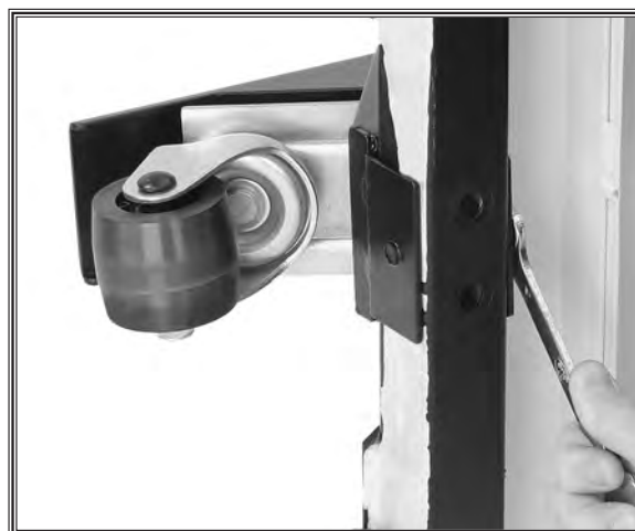
Figure 9. Bolting wheel assembly to stand.
