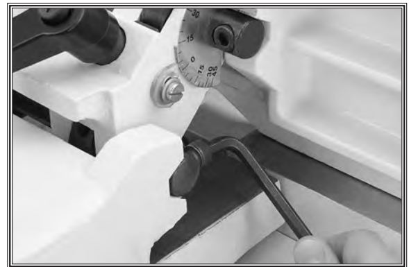
Figure 20. Attaching fence to carriage.
