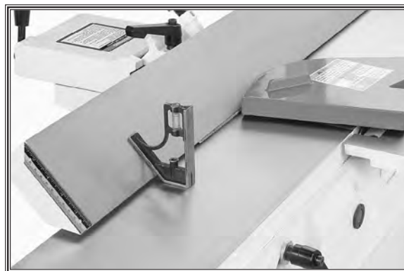
Figure 63. Adjusting fence 45° outward.
