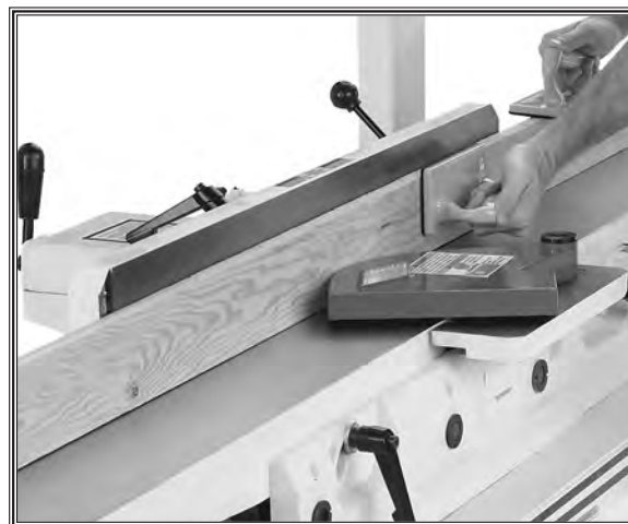
Figure 38. Typical edge jointing operation.
