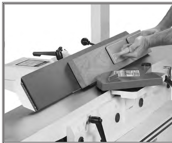
Figure 40. Typical bevel cutting operation.
