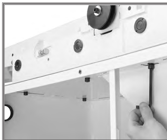
Figure 11. Securing the jointer to the stand.
