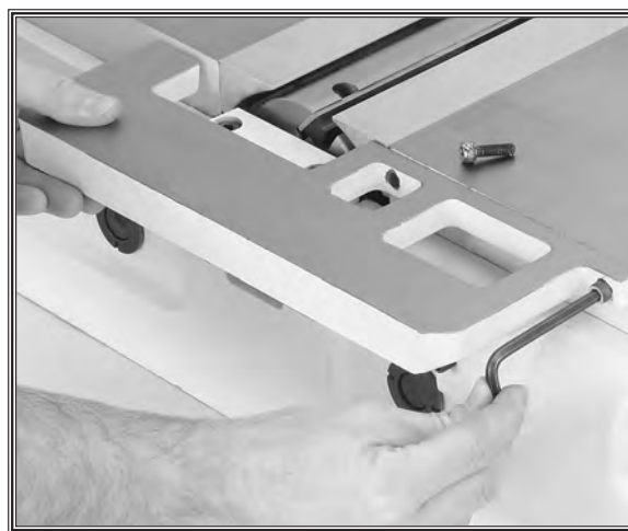
Figure 16. Attaching extension table to jointer.
