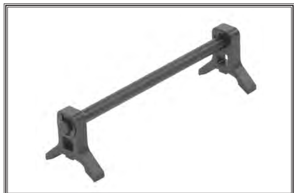
Figure 25. Knife setting jig assembly.
