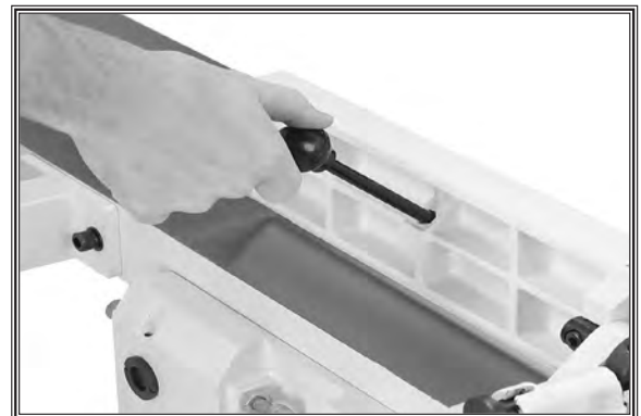
Figure 21. Installing the tilt lever.
