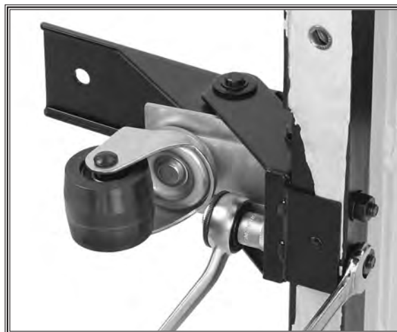
Figure 10. Securing wheel assembly to stand.
