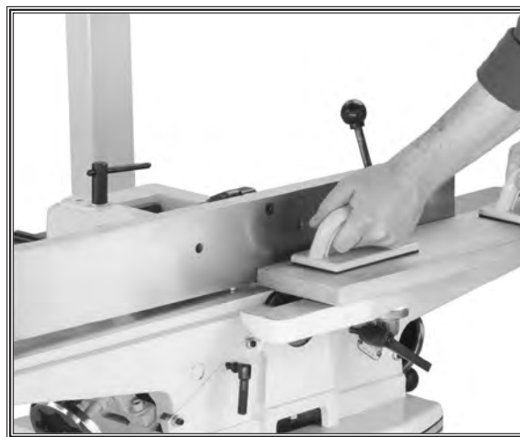
Figure 42. Typical rabbet cutting operation.
