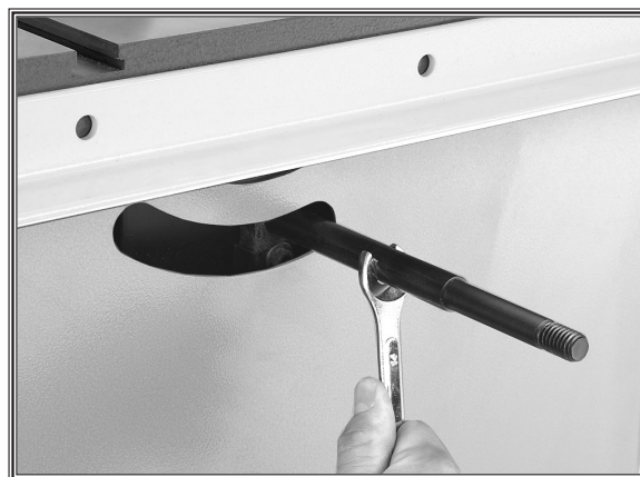
Figure 12. Installing the pivot shaft.
