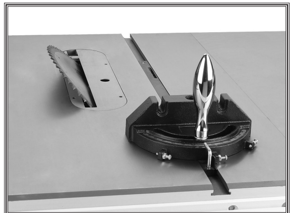
Figure 25. Blade tilted to 45° (guard removed for clarity).
