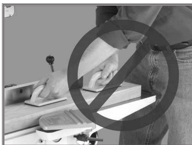
Figure 5. Never stand directly behind the workpiece!
