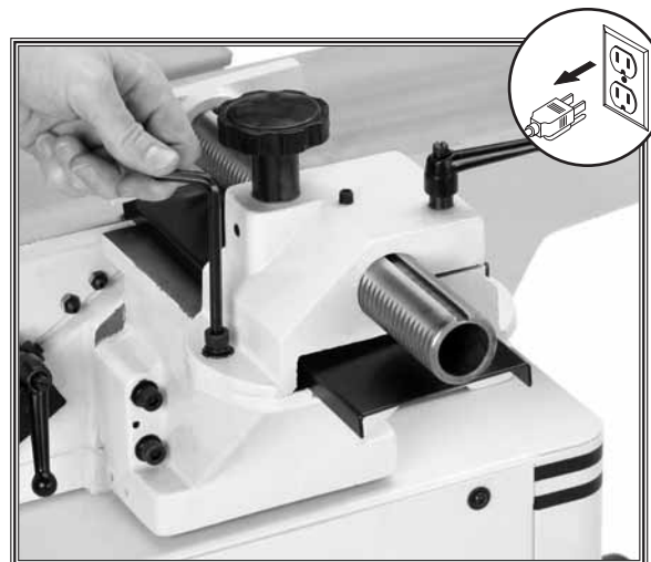
Figure 19. Fence carriage assembly.
