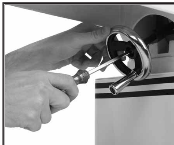
Figure 28. Securing the handwheel.
