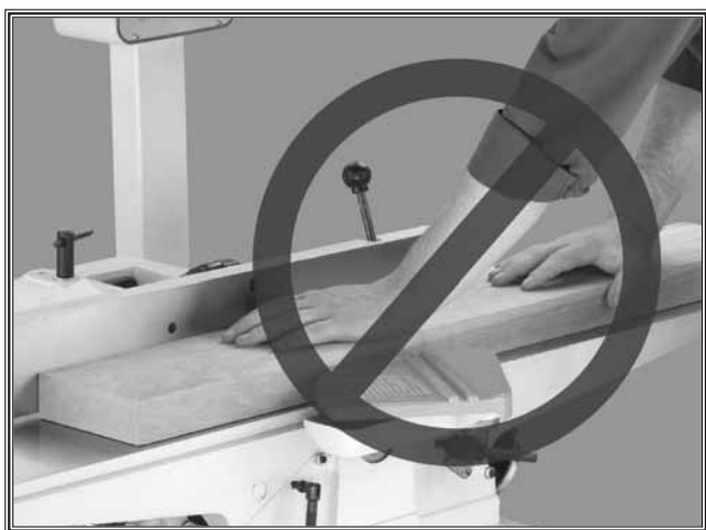
Figure 3. Never surface plane without push-blocks!
