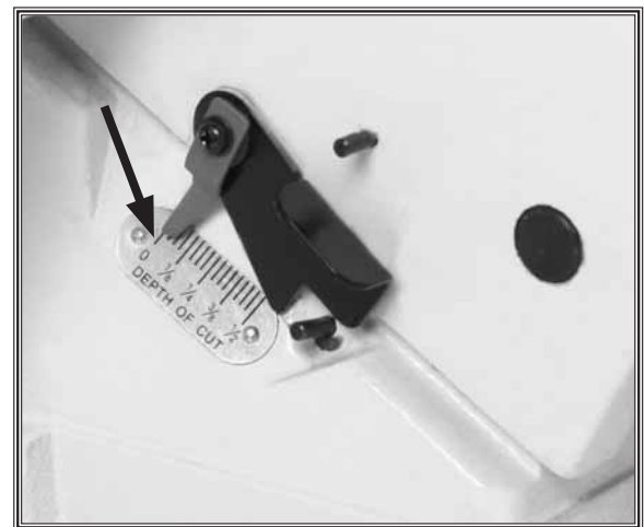
Figure 54. Depth-of-cut pointer adjusted to "0" position.
