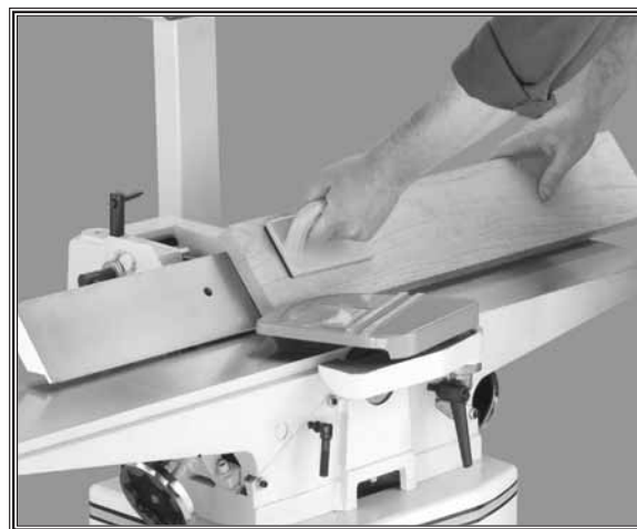
Figure 46. Typical bevel cutting operation.
