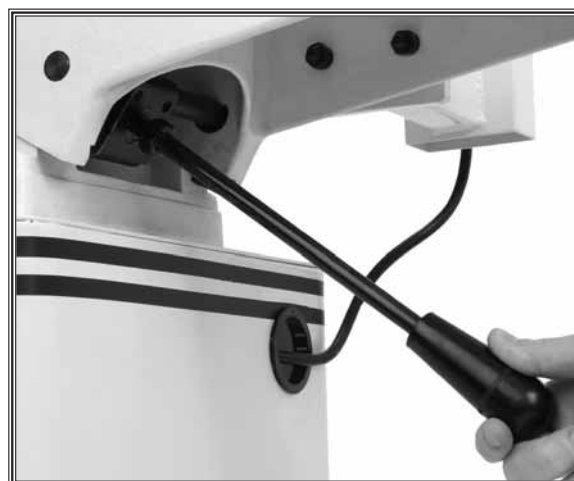
Figure 29. Installing infeed table lever.
