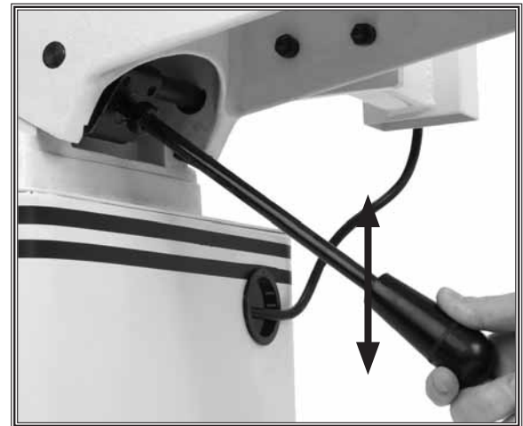
Figure 34. Adjusting infeed table height.
