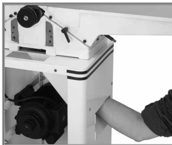
Figure 14. Installing forward mounting bolt.
