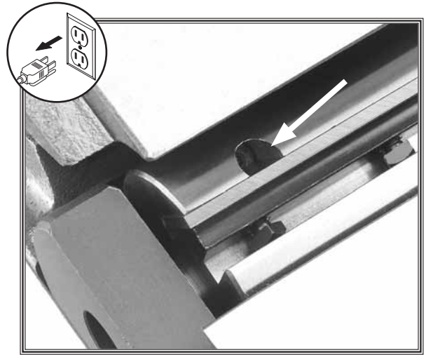
Figure 52. Jack screw access hole.
