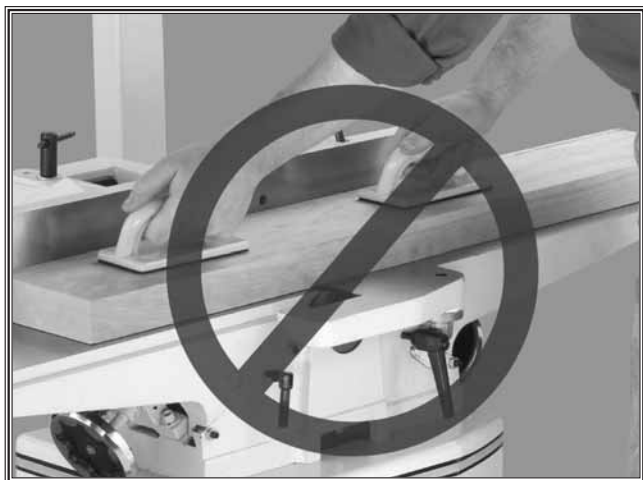
Figure 4. Never plane/edge-joint with the guard removed!
