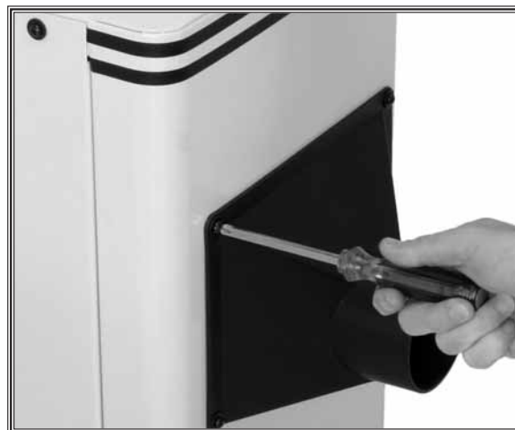
Figure 25. Dust port installation.
