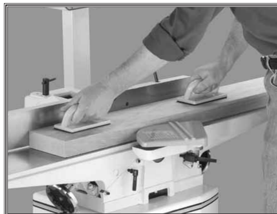
Figure 42. Typical surface planing operation.
