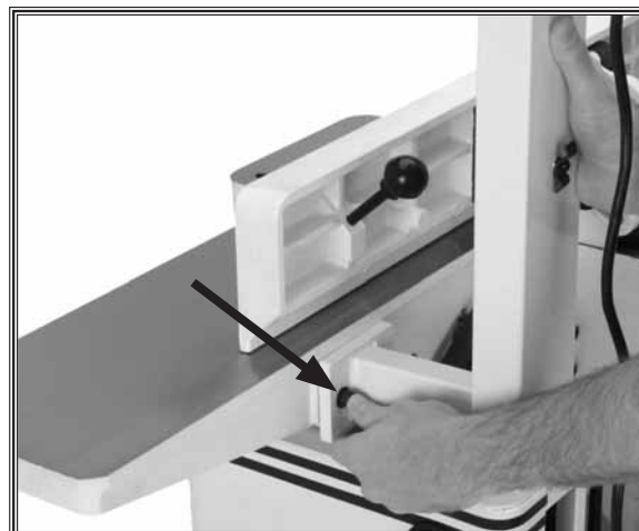
Figure 26. Installing support arm.
