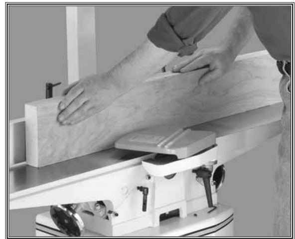
Figure 44. Typical edge jointing operation.
