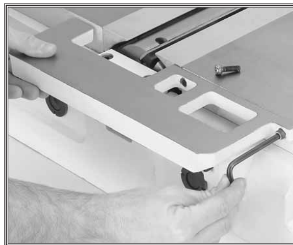
Figure 15. Attaching extension table to jointer.
