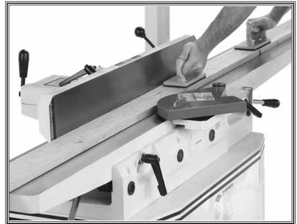
Figure 34. Typical surface planing operation.
