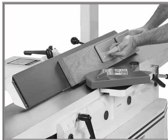
Figure 38. Typical bevel cutting operation.
