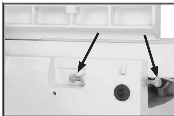
Figure 46. Table positive stop bolts.
