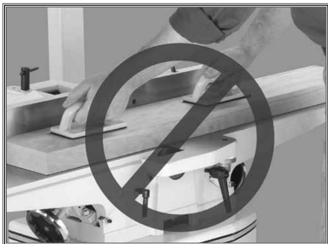
Figure 3. Never plane/edge-joint with the guard removed!
