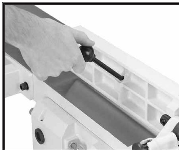
Figure 19. Installing the tilt lever.
