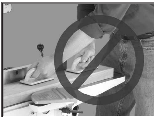
Figure 4. Never stand directly behind the workpiece!
