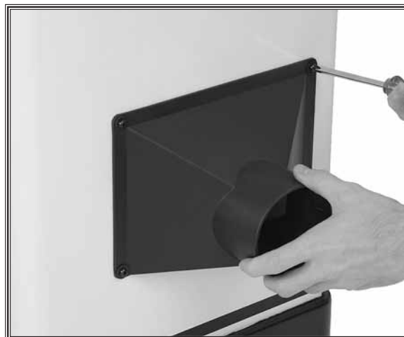
Figure 22. Attaching dust port to jointer stand.
