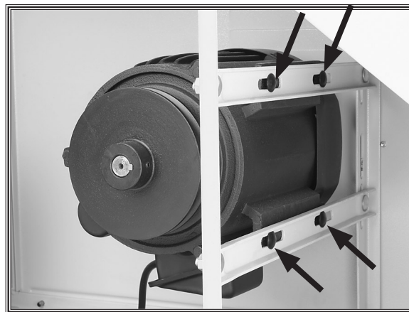
Figure 2. Motor attached to the motor mounts.
