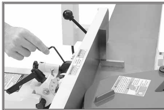
Figure 58. Adjusting fence to 90°.
