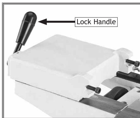
Figure 17. Fence carriage mounted on the back of the jointer.
