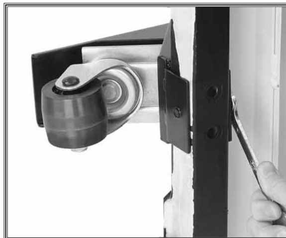
Figure 9. Bolting wheel assembly to stand.
