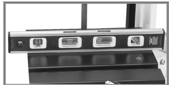
Figure 23. Adjusting table with a level.
