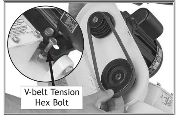
**Figure 14.** Installing the V-belt.
