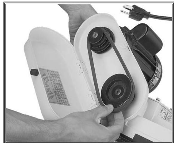
**Figure 50.** Installing the V-belt.
