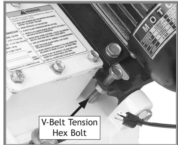
**Figure 49.** V-belt tension hex bolt.
