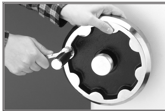
Figure 22. Installing handwheel, lock knob and handle.
