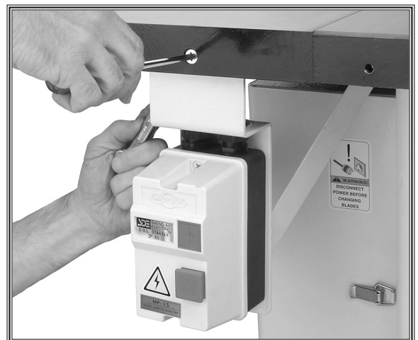
Figure 20. Attaching switch to extension wing.
