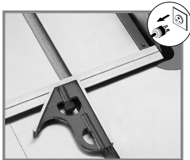
Figure 66. Measuring blade to miter slot.
