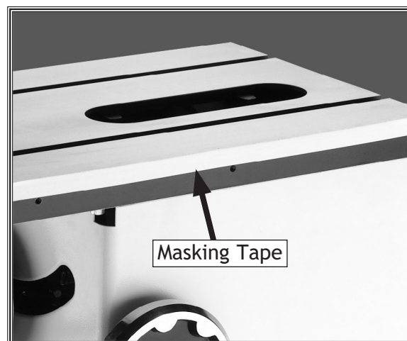
Figure 70. Shimming table with masking tape.
