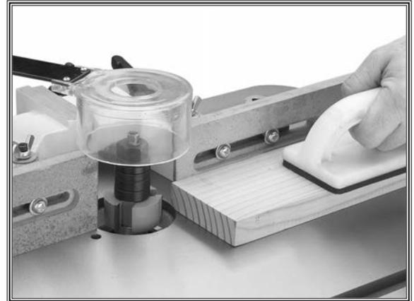
Figure 16. Shaper cutter installed on spindle.
