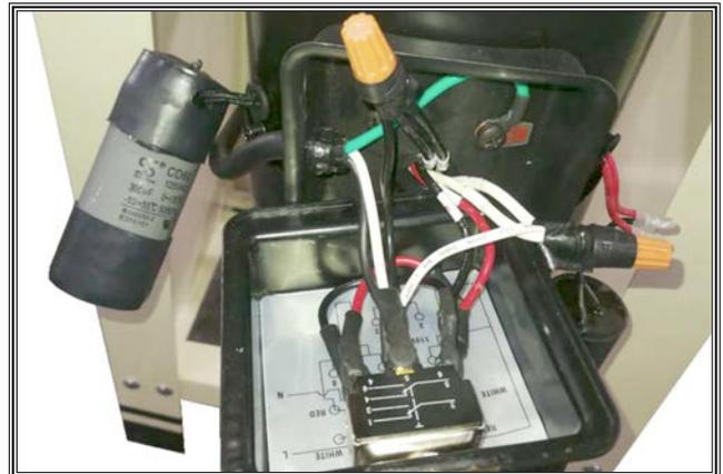
Figure 60. Motor and FOR/REV switch.
