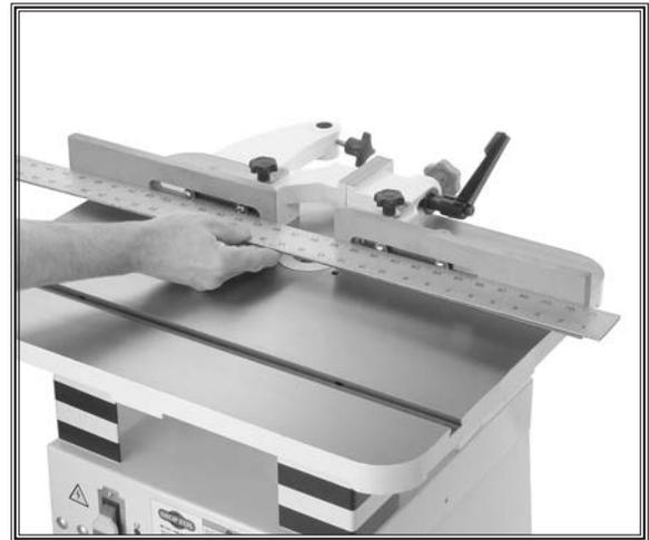
**Figure 22.** Use straightedge to check fence.
