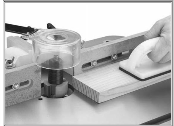
Figure 16. Shaper cutter installed on spindle.
