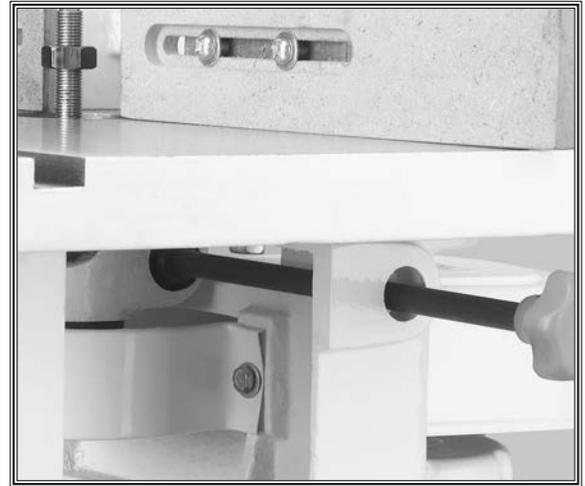
Figure 18. Spindle lock knob.
