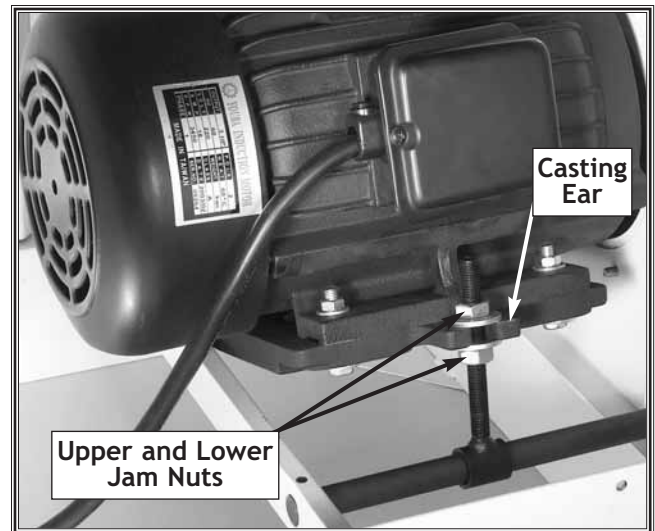
Figure 40. V-belt adjustment jam nut.
