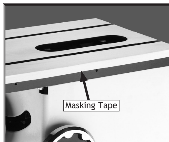
Figure 70. Shimming table with masking tape.
