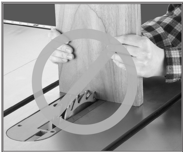
Figure 7. Do not make unstable cuts.
