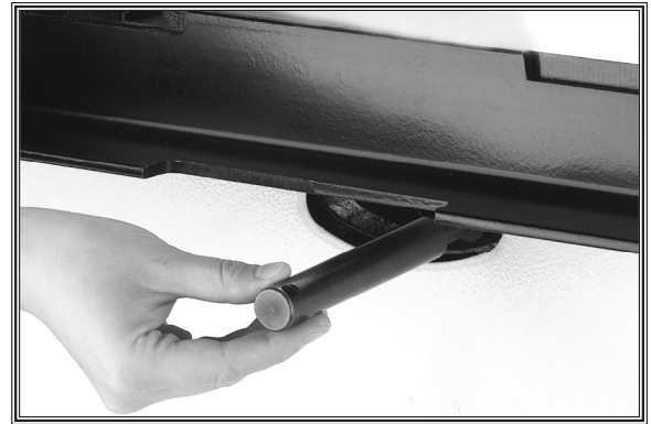
Figure 26. Installing the splitter shaft.
