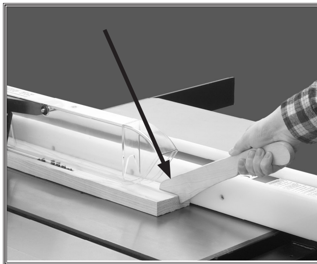
Figure 9. Use a push stick when ripping narrow pieces.
