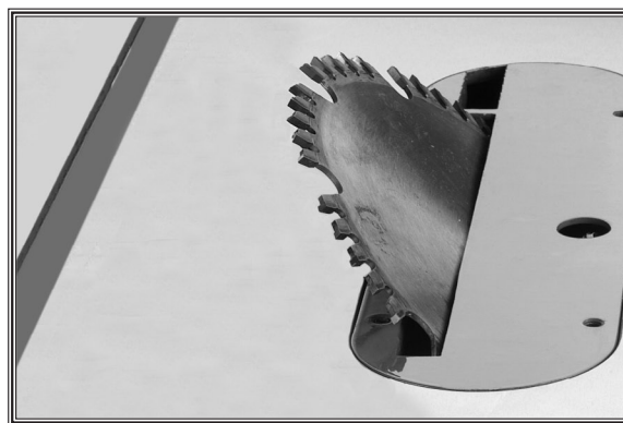
Figure 41. Blade tilted to 45° (guard removed for photo clarity).
