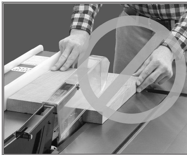
Figure 10. Do not stand directly behind blade when making a cut.
