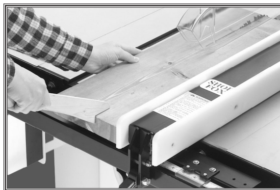
Figure 40. Typical rip cut.
