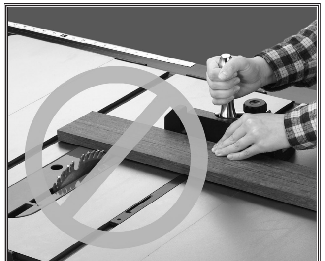
Figure 6. Do not make through cuts without the blade guard/splitter in place.
