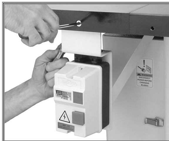
Figure 20. Attaching switch to extension wing.
