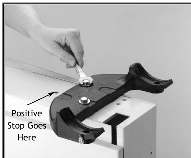
Figure 17. Attaching trunnion support to body.
