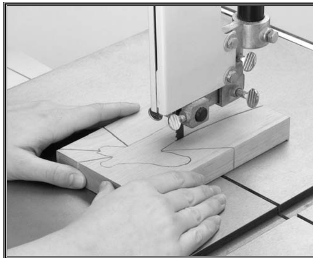
Figure 9. Use relief cuts for tight curves.
