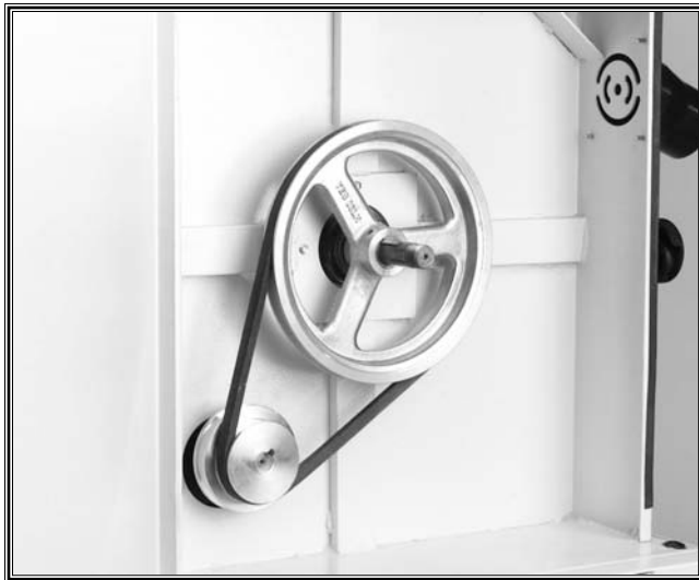
Figure 28. Speed pulley (lower wheel removed for clarity).
