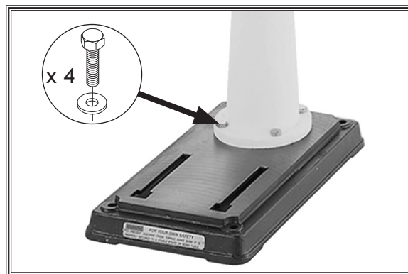
Figure 11. Column secured to base.
