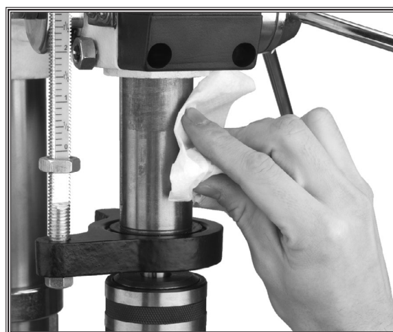
Figure 45. Clean and oil quill shaft.
