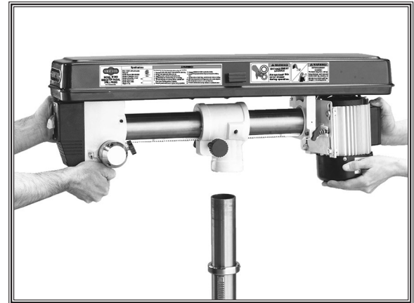
Figure 19. Installing the headstock onto the column.
