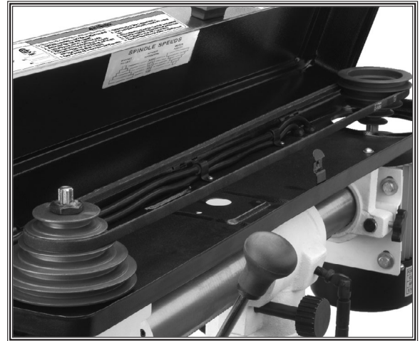
Figure 38. Belt safety cover opened.
