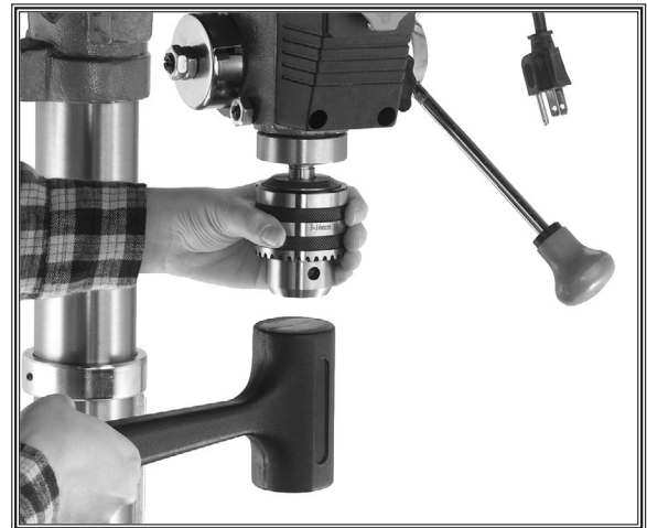
Figure 24. Example of joining drill chuck to arbor.
