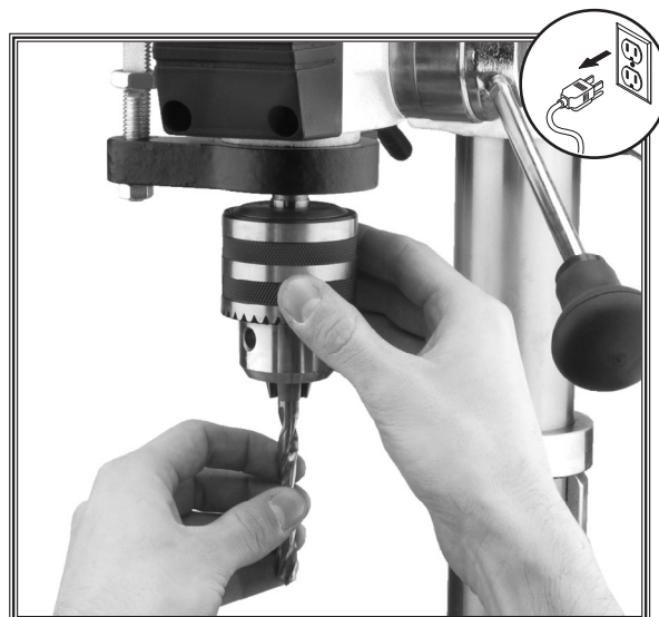
Figure 29. Installing a drill bit.
