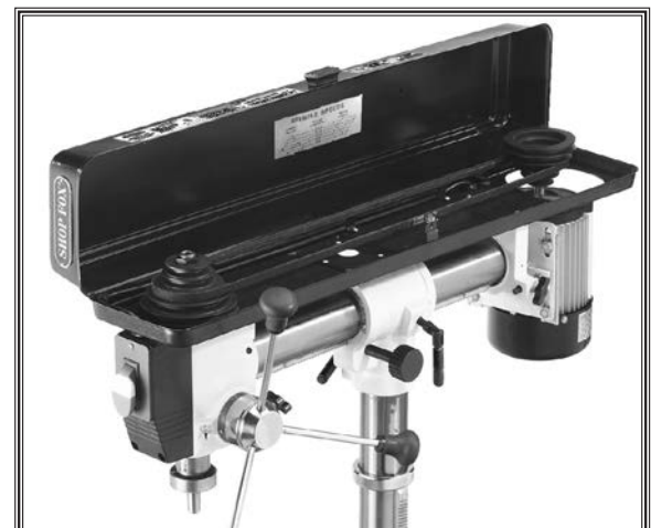
Figure 28. Belt set to desired speed.
