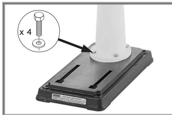
Figure 11. Column secured to base.
