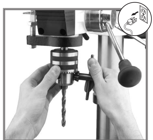
Figure 30. Using the chuck key.
