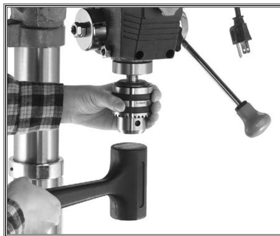
Figure 24. Example of joining drill chuck to arbor.
