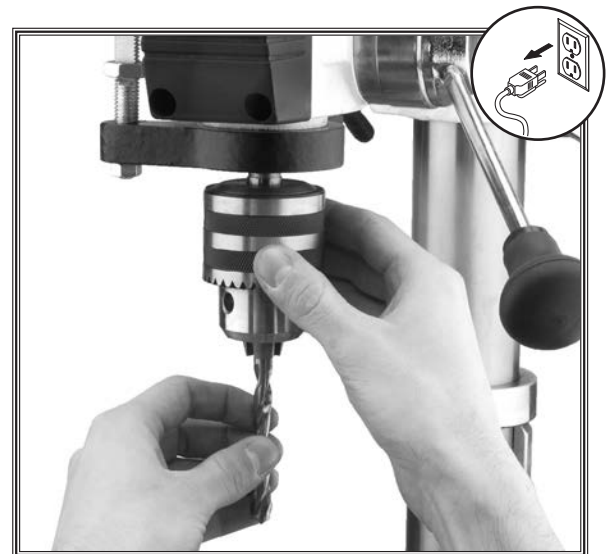
Figure 29. Installing a drill bit.
