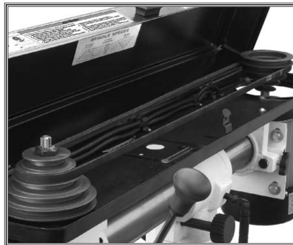
Figure 38. Belt safety cover opened.
