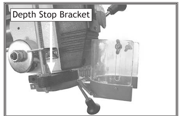
Figure 22. Chuck guard installed on depth stop bracket.
