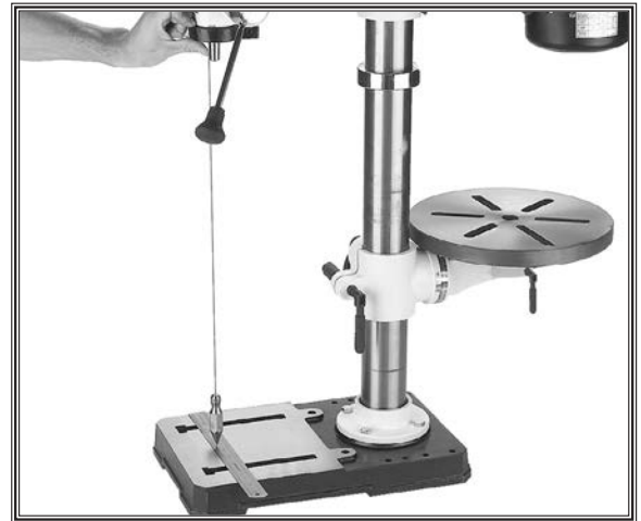
Figure 21. Aligning the headstock.
