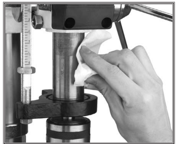
Figure 45. Clean and oil quill shaft.
