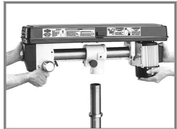
Figure 19. Installing the headstock onto the column.
