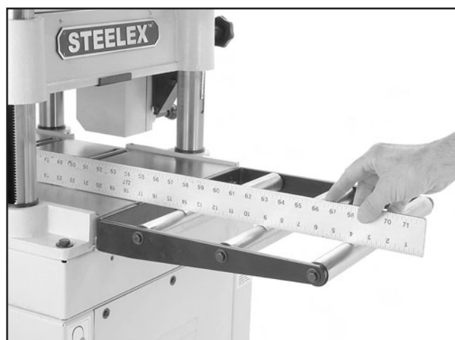
Figure 14. Checking table-extension roller alignment.
