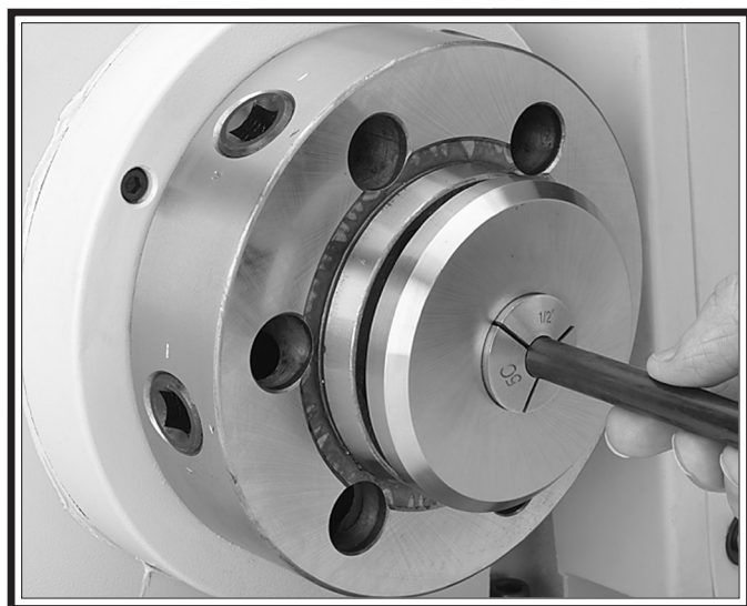
Figure 11. Installing a workpiece.
