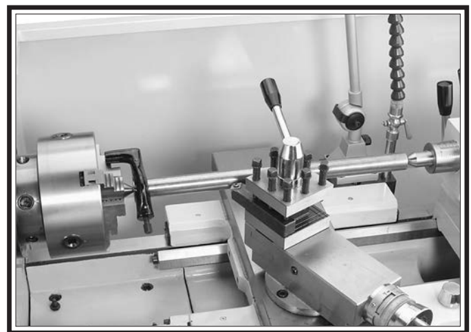
Figure 50. Example photo of a workpiece mounted between the centers.
