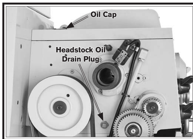
Figure 99. Headstock oil cap and drain plug.
