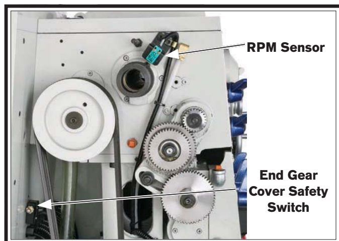
Figure 146. End gear cover safety switch and RPM sensor.
