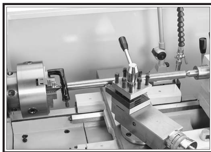
Figure 53. Example photo of a workpiece mounted between the centers.
