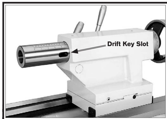
Figure 52. Drift key slot in the side of the quill.
