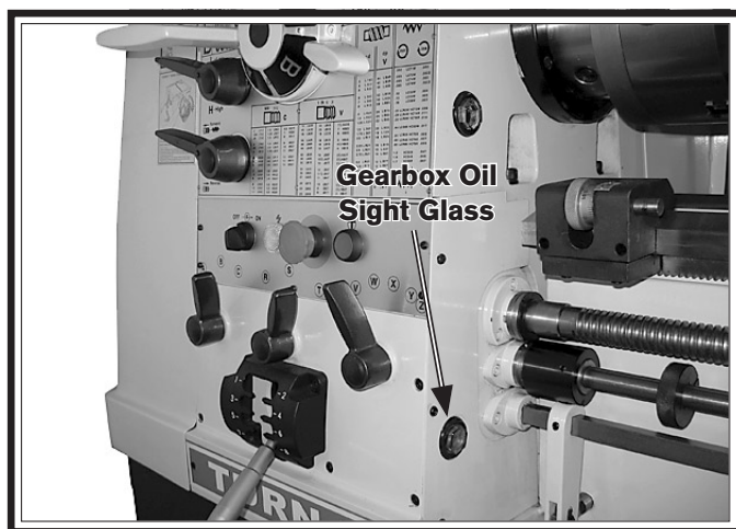
Figure 102. Location of quick-change gearbox oil sight glass.
