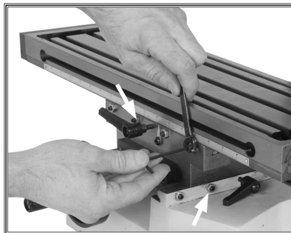
Figure 29. Gib screws and adjustment.
