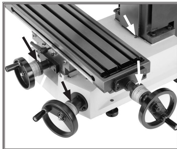
Figure 27. Table and base ball oiler locations.
