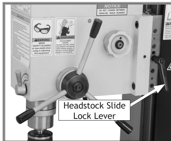
Figure 14. Headstock slide controls.
