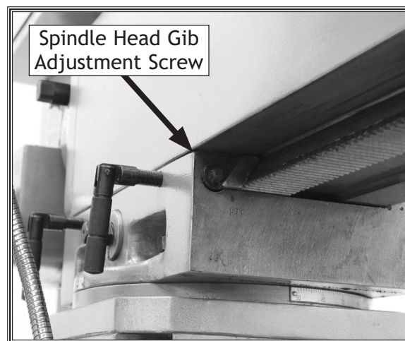
Figure 49. Location of end of spindle head gib adjustment screw.
