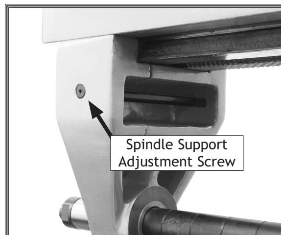
Figure 50. Location of adjustment screw for spindle support dovetail clamp.
