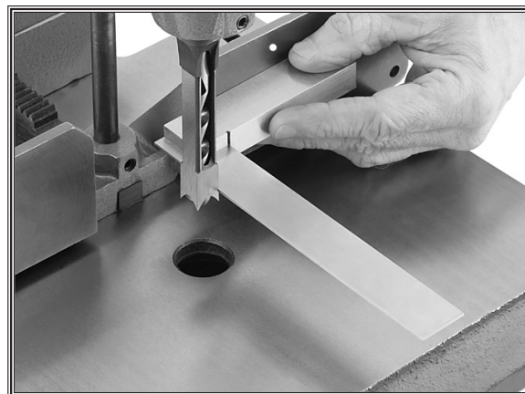
Figure 5. Example of squaring a chisel.
