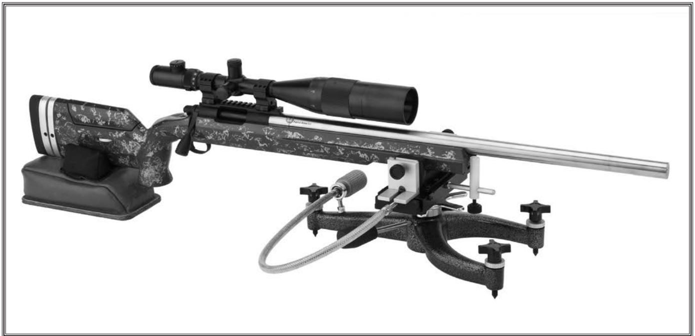
Figure 15. Overview of an example rifle setup on the windage shooting rest (BE1005 shown).
